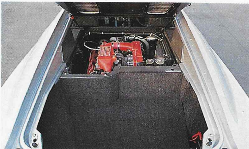
264bhp 2.2-litre four is as potent as ever
